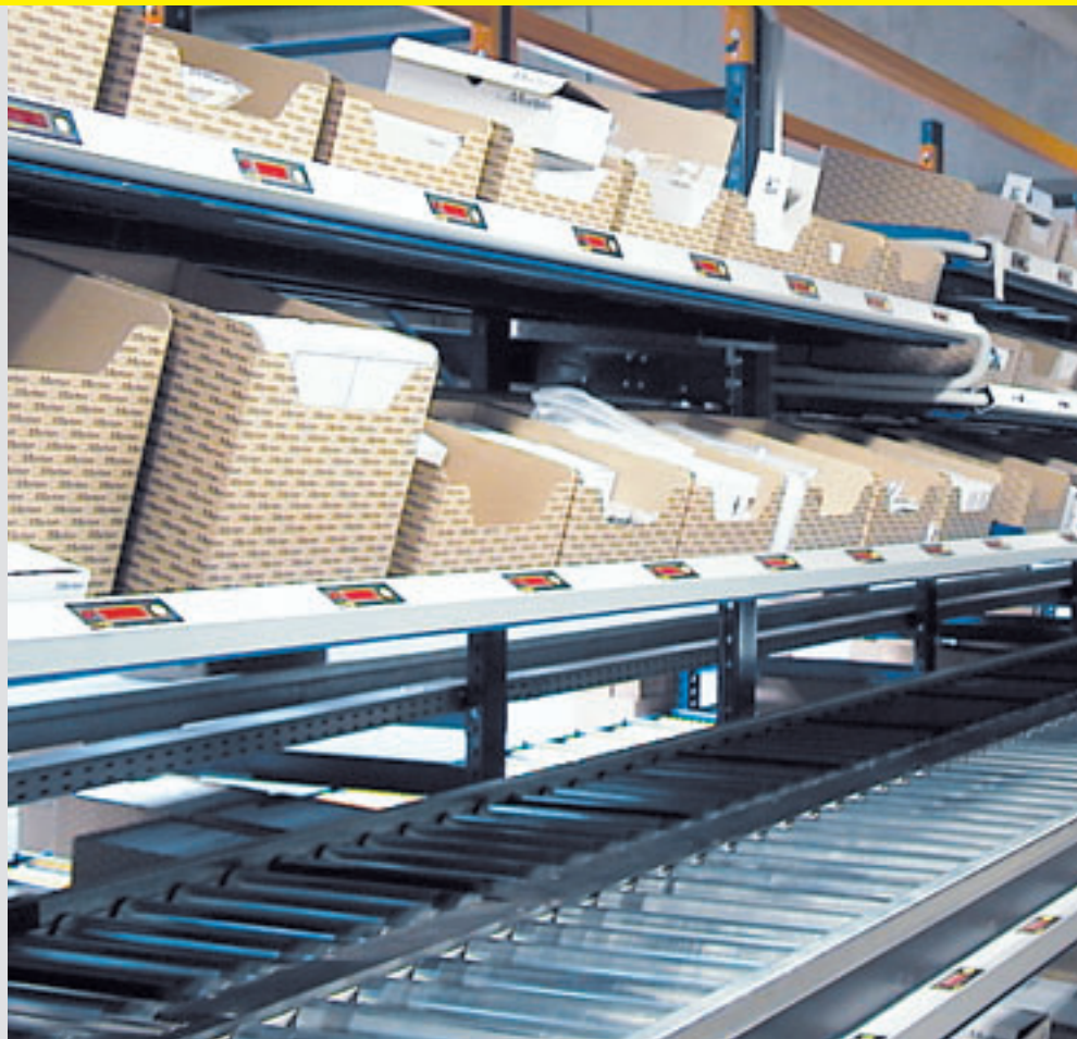
Illustration bottom: Pick-by-light reduces the error rate and increases the picking speed in the electronics industry
