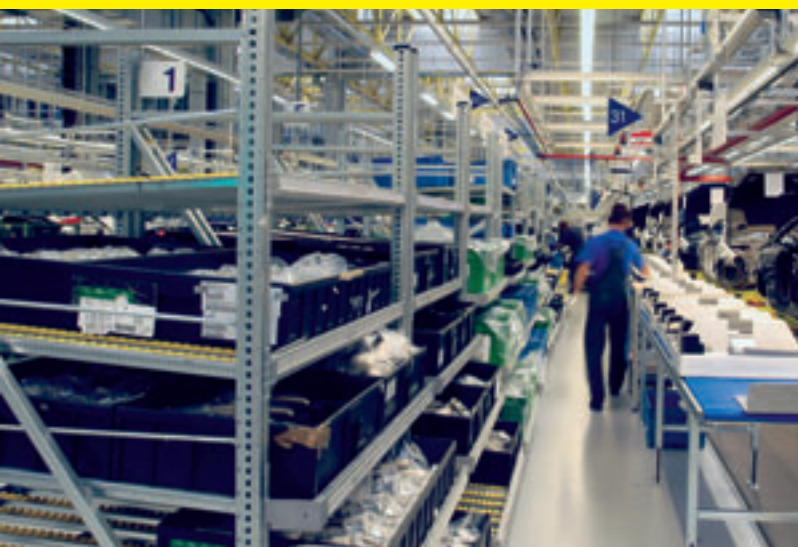
R 7000 on-line shelving with glide rails
