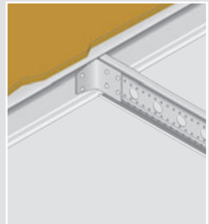
Platform supports made from a combination of hot rolled steel profiles and system profiles
