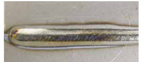
Copper – plasma-melt in 0.6 mm wall thickness
