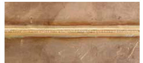
Copper – plasma-melt in 0.6 mm wall thickness
