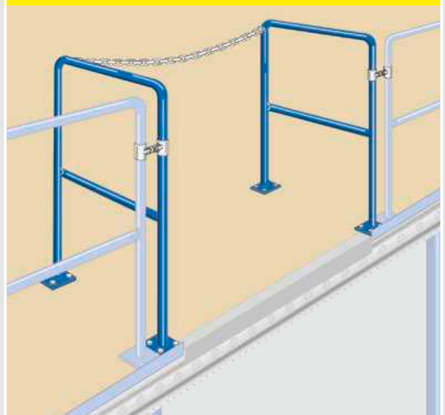
Transfer position with chain barrier
